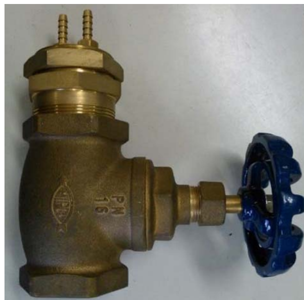
Fig. 8. Adapter coupled to the valve 2".
